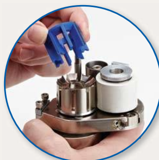
Remove used blade cartridge
