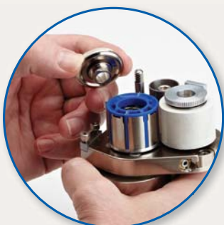
Remove locking mechanism
